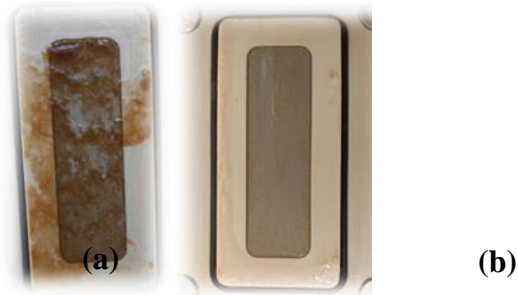
Figure 7: Ultrasonic device heating surface before (a) and after (b) the biocide dosage strategy change.
